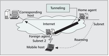
**Figure 1.** *Mobile IPv4 architecture.*
