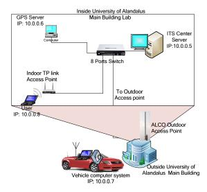
Figure 4: System testbed and components
