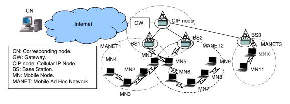
Figure1: Integrated network architecture.
